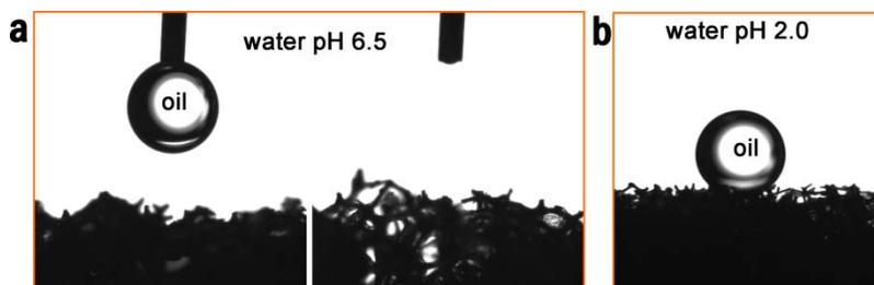
**Figure S3. a**, Still images from video CA measurements of a DCE droplet on the functionalized sponge in water with a pH of 6.5. Upon contacting, the oil droplet was quickly sucked up by the sponge, indicating the superoleophilicity. **b**, Image of a DCE droplet applied on the surface of the functionalized sponge in water with a pH of 2.0, showing the superoleophobicity of the surface in the acidic water.
