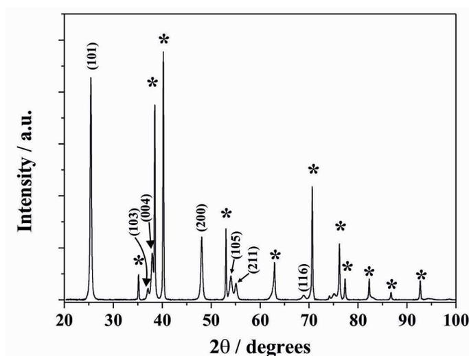
**Figure S1.** XRD pattern of TiO<sub>2</sub> NTs annealed at 450 °C for 1h.
