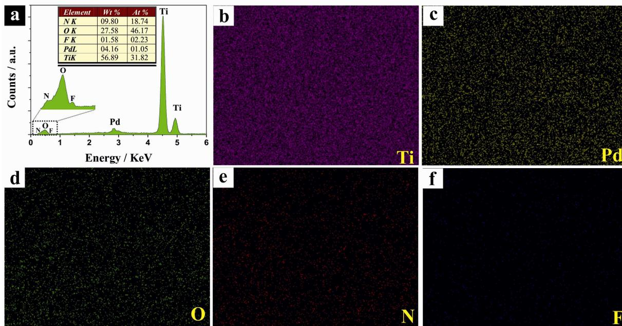
**Figure S2.** (a) EDX spectrum of Pd/TiO<sub>2</sub> NTs; EDX elemental mapping of (b) Ti, (c) Pd, (d) O, (e) N, and (f) F on the top surface.
